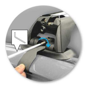
• Tighten adjusting screw to 5 Nm (3.7 ft lb).
